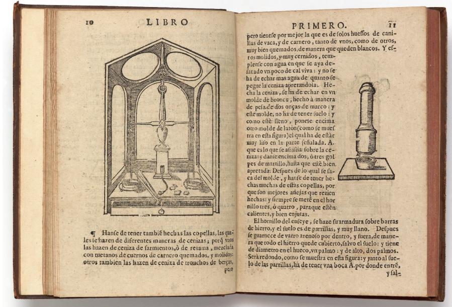
Precision balance for the weighing of precious metals and stones (page height 200 mm)
